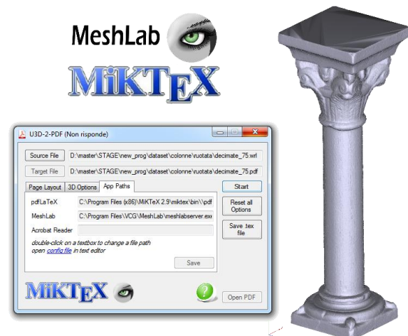
Fig. 15: Open Source pipeline for generating 3DPDF: the resulting model loses information and color segmentation, but takes advantage of the considerable compression of the U3D model (software: U3D2PDF - MeshLab+MiKTeX).
