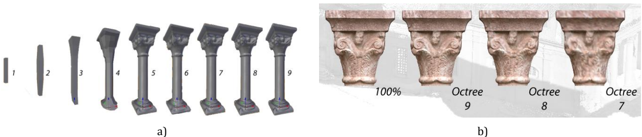
Fig. 11: Two examples of Remesh simplification with different values of octree (software: Blender 2.68, comand: Remesh - Marching Cubes).
