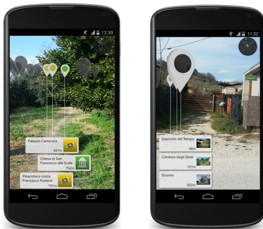
Fig. 5: The mobile application running during the visit of Cardeto Park. The Points of Interest are shown once the user get into the pre-defined area of influence of any attraction.
