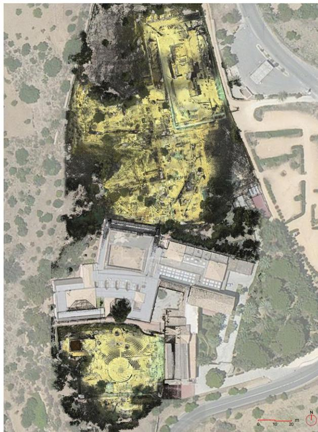
**Fig. 2:** *Upper Agora*. Planimetric orthoprojection of the point cloud model overlapped on the ortho-photo
