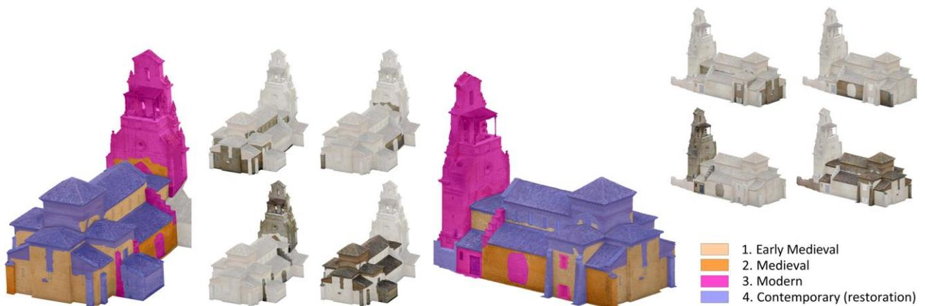
Fig. 12: Visualization of the evolution of the building through its 3D model
