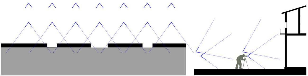
**Fig. 9:** Shooting with parallel axes (simple or multiple)
