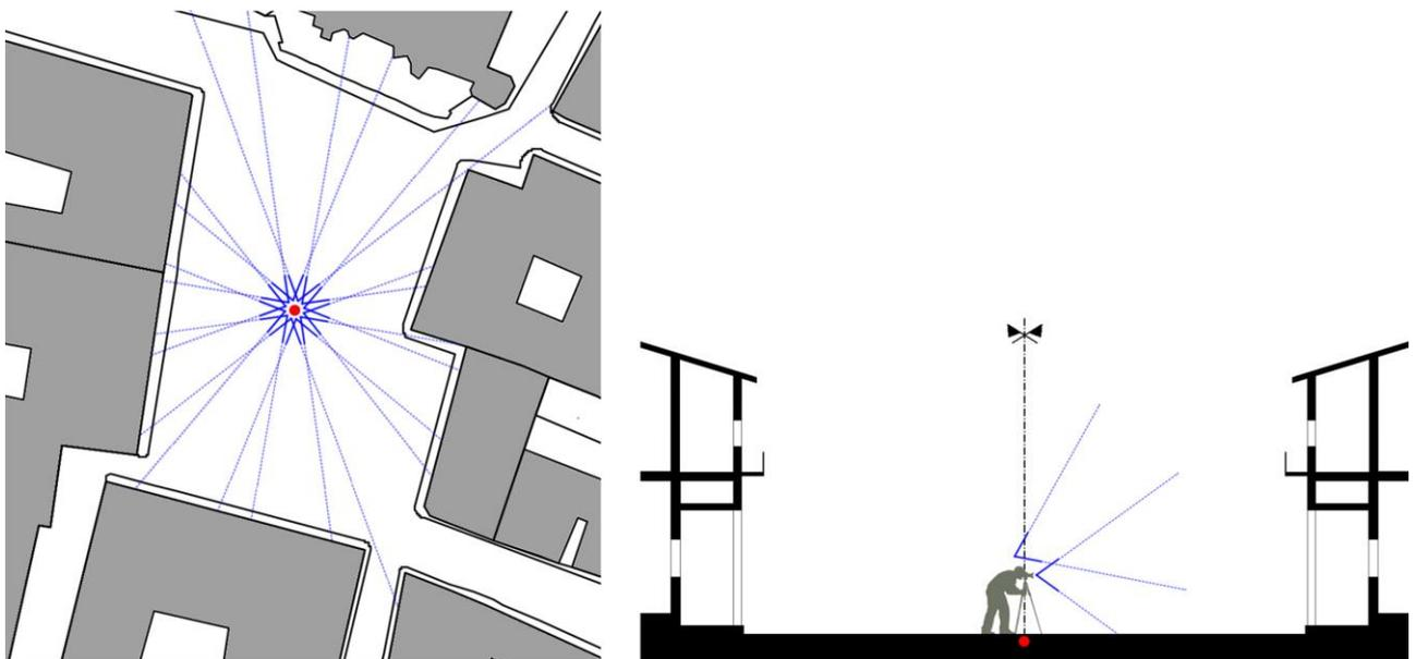
**Fig. 11:** Panoramic shooting (cylindrical, spherical or partial)
