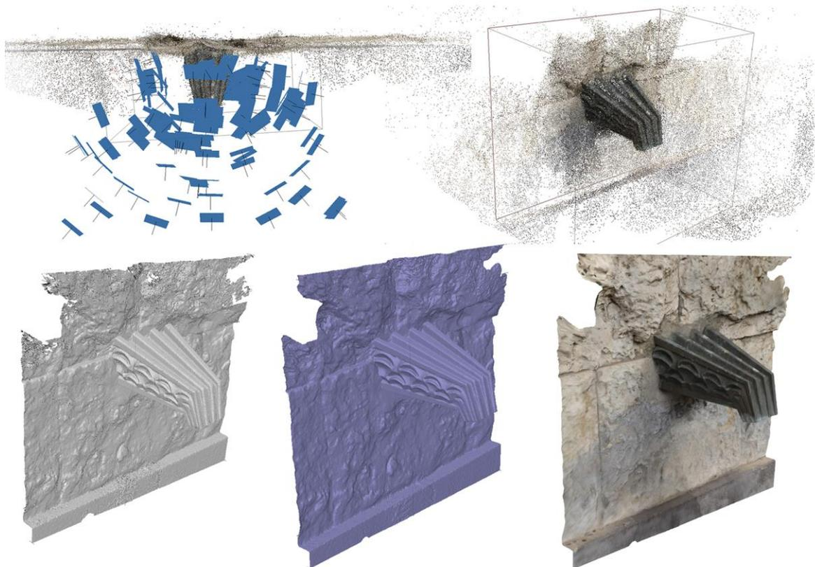
Fig. 3: INPS building: Structure from Motion of detail
