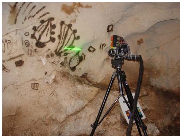
Fig. 10: Multi-resolution 3D model of a section of the cave with a series of pictograms - photograph of close range scanner, (3D laser scanner 2005).
