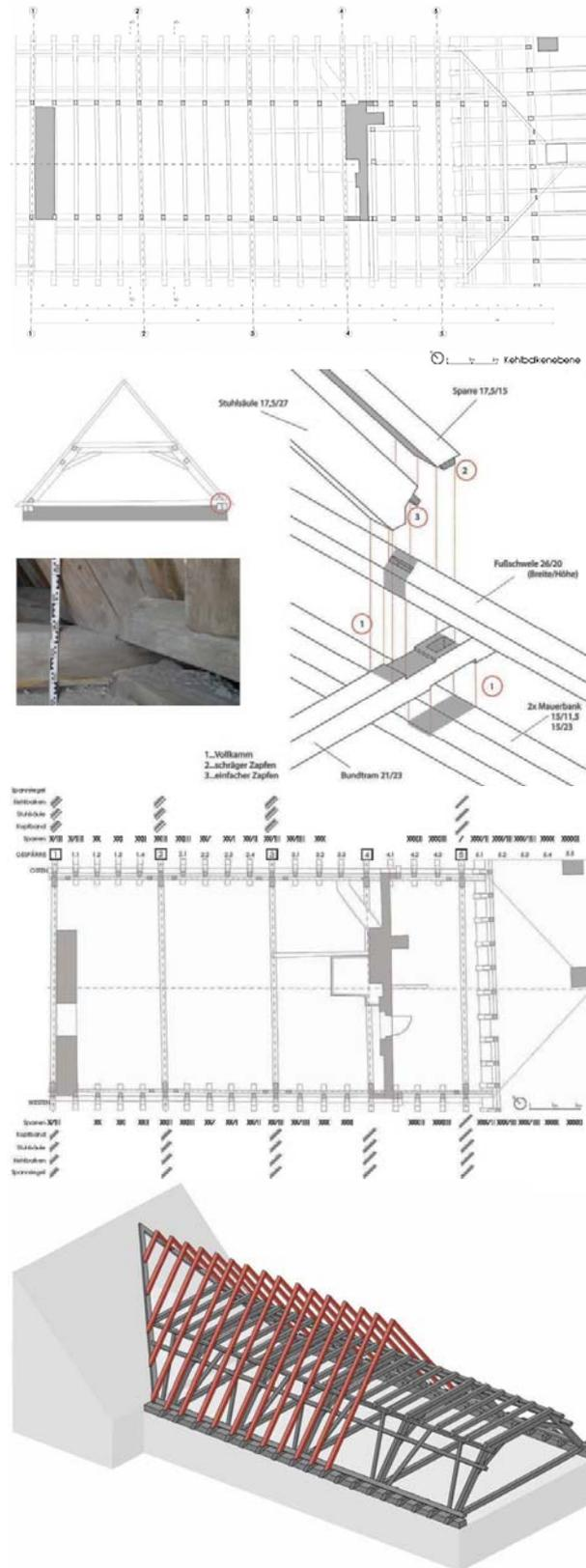
Fig. 1: Results of the architectural analysis of historic roof structures: survey plans, details of joints, carpenter`s marks, hypothesis on the process of assembly (E. G. Gürbüz, V. Hristova, M. Obermoser, A. Seeber; all TU Wien, 2016)
