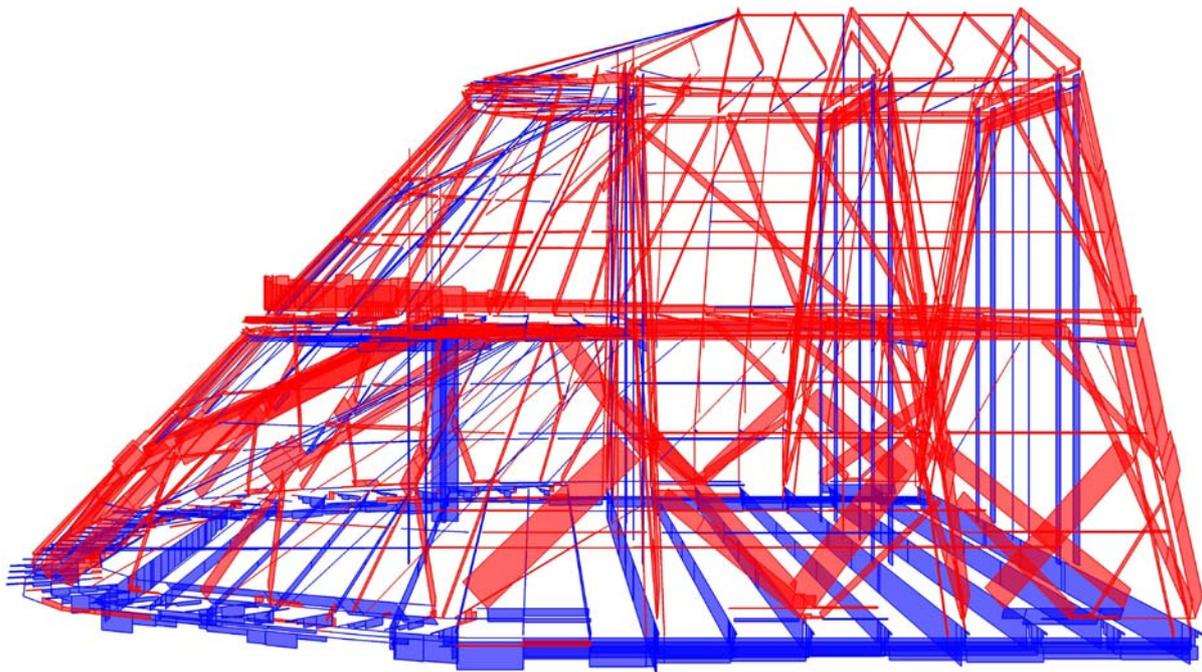
**Fig. 5:** Distribution of normal forces depending on the structural characteristic of step joints. Roof structure of the Spanish Riding School in the Vienna Hofburg G. Hochreiner, TU Wien 2019
