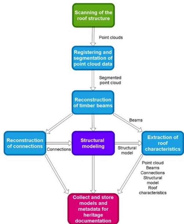
Fig. 3: Main process workflow from point cloud to BIM documentation (T. Özkan, TU Wien 2020)
