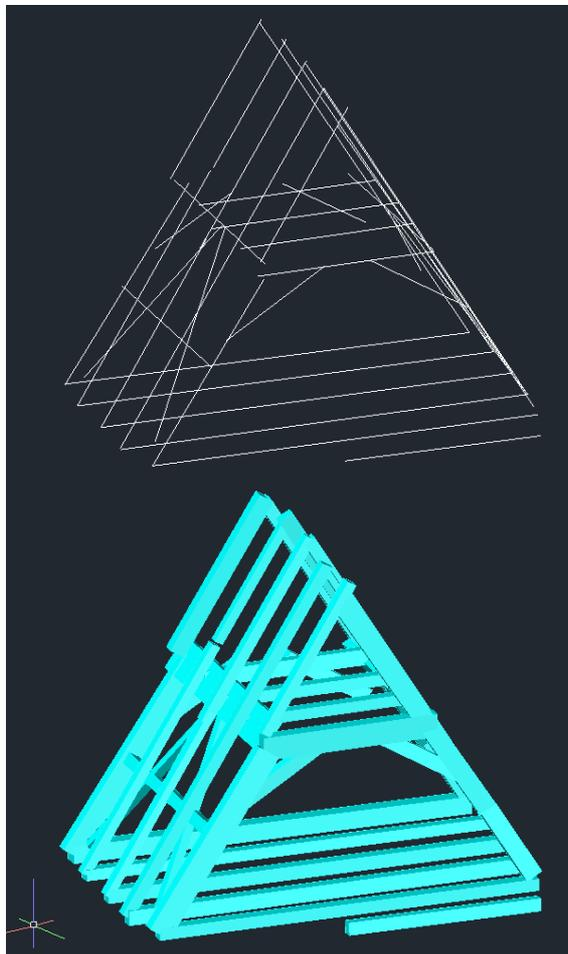
**Fig. 4:** Reconstructed roof structure of the Amalienburg in the Vienna Hofburg. Top: Central axes of beams. Bottom: cuboid representation (M. Pöchtrager, TU Wien 2018)
