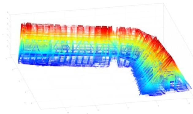
**Fig. 2:** Roof structure of the Amalienburg in the Vienna Hofburg, 3D point cloud (T. Mittrecker and M. Pöchtrager, TU Wien 2017)
