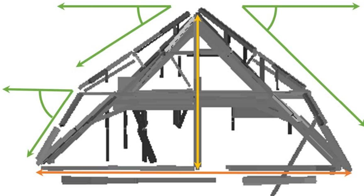
**Fig. 6:** Derivation of further architectural roof characteristics. Southern wing of the Austrian National Library (M. Pöchtrager, TU Wien 2018)
