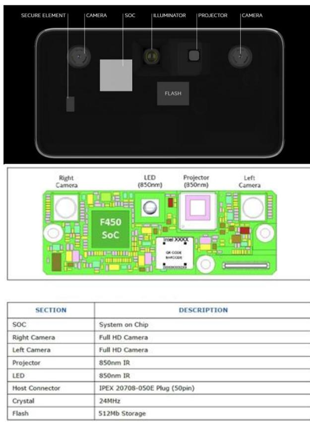
Fig. 3: Intel RealSense solution, module and component list
