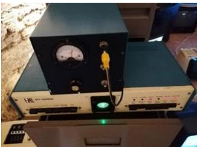
Fig. 10: Modem and power supply for Olivetti teletype
