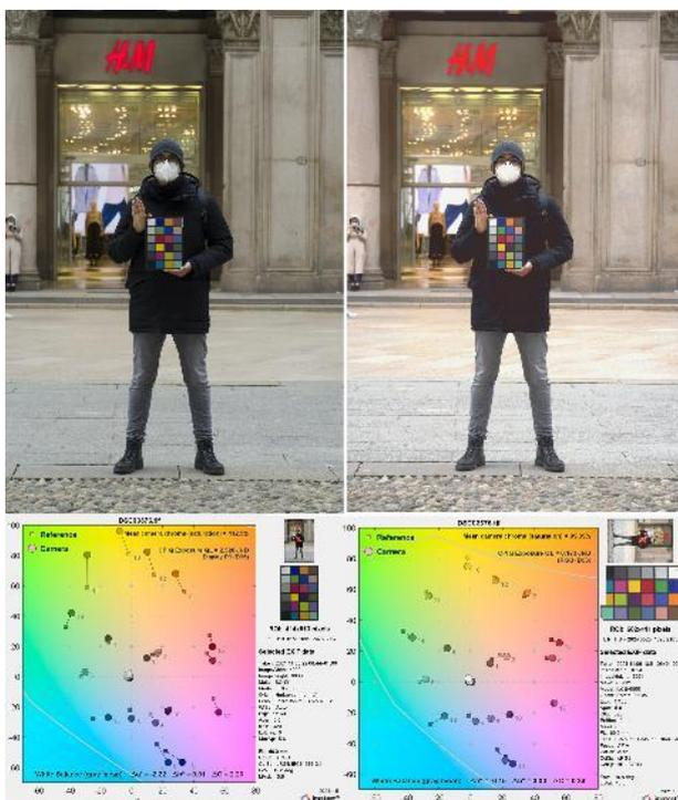
Fig. 4: Color corrected images: on the left using a manual correction (error  $\Delta E_{00} \text{ mean} = 11,31$ ); on the right using the SHAFT software (error  $\Delta E_{00} \text{ mean} = 2,04$ ).
