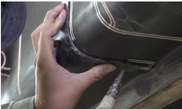
Fig. 15: Outline the raised pattern through the tip of the tube stuffed with the paste
