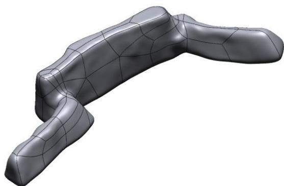
**Fig. 13:** Closed surface generated from the mesh in MeshLab. Geomagic Design X
