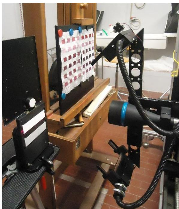
**Fig. 1:** IFAC-CNR spectrographic imaging head with the lighting module during the acquisition of HSI data.
