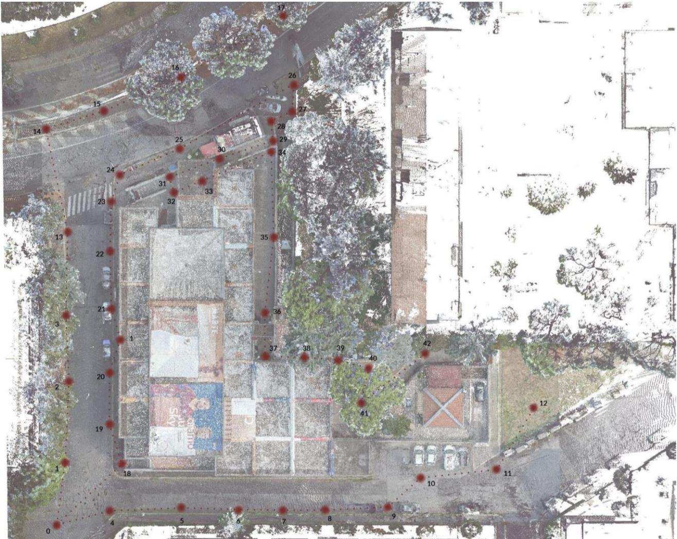
**Fig. 4:** Complete cloud of points obtained by laser scanners and UAVs in which the station points of the laser scanner are indicated (graphic elaboration by the authors).
