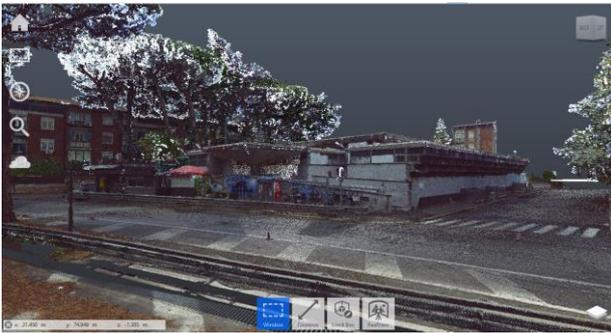
**Fig. 5:** Walls of the Ex Mercato di Torre Spaccata with the closures added in the 1980s: metric data and RGB data of the point cloud obtained by laser scanners.
