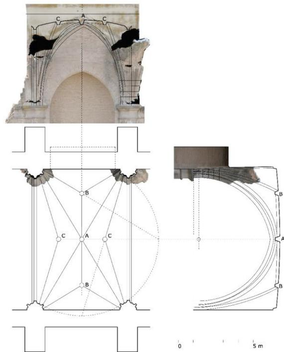
Fig. 17: Geometric framework of a vault based on the orthogonal projections of the scanned *tas-de-charges*
