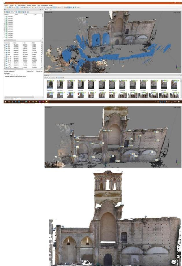
**Fig. 3:** Photogrammetry workflow: orientation of the photographs, control points and orthophotograph generated.
