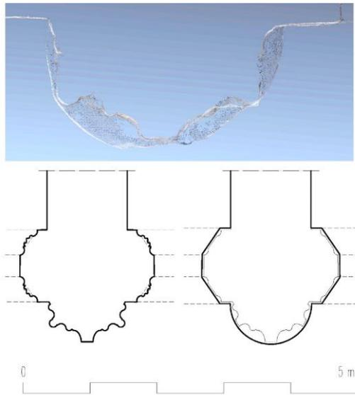
**Fig. 5:** Orthophoto of the photogrammetry of the pilasters and floor plans of the state before and after the Renaissance adaptation.
