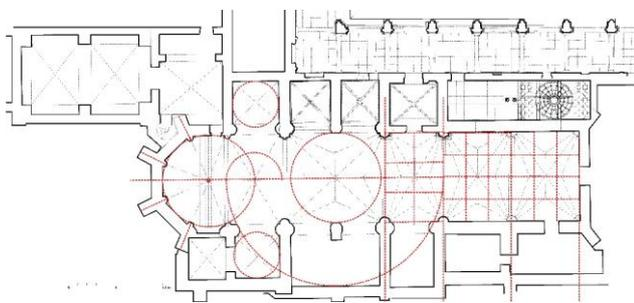
Fig. 16: Geometric framework of the church floor plan
