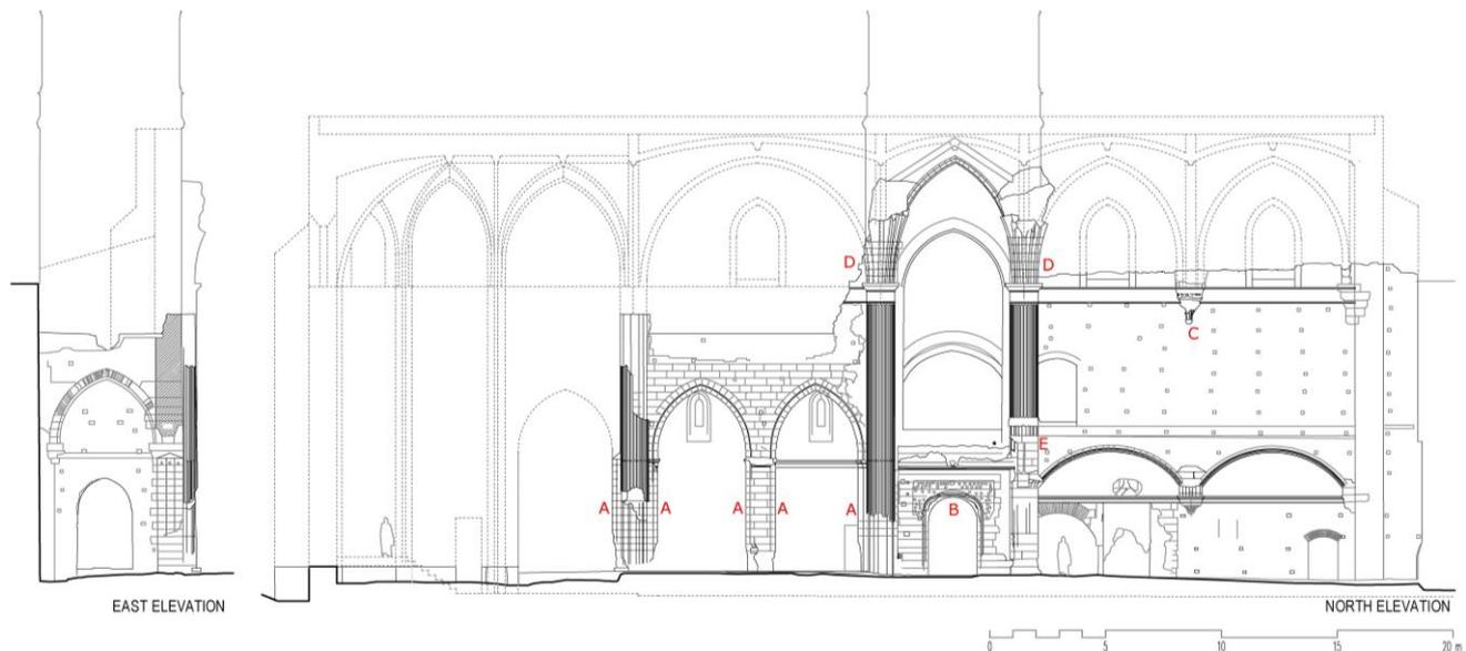
**Fig. 4:** Elevation indicating inventoried elements
