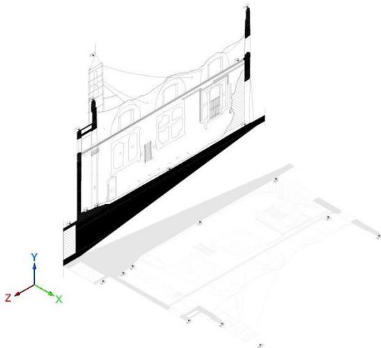
**Fig. 3:** Import from AutoCAD longitudinal section to Autodesk Revit project.
