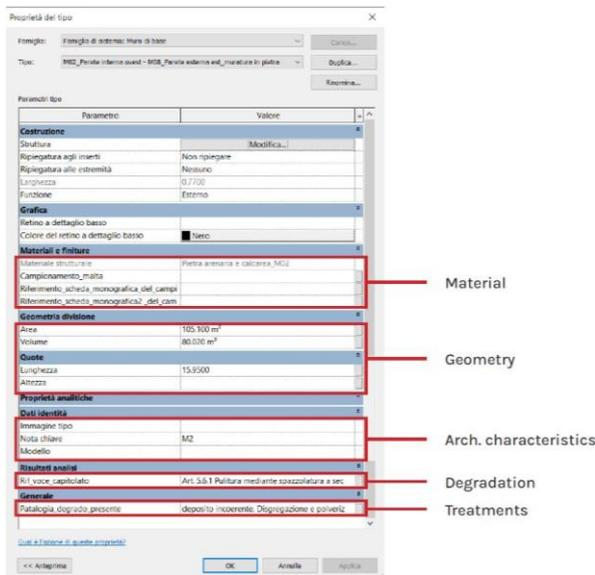
Fig. 6: Parameters of a generic system family
