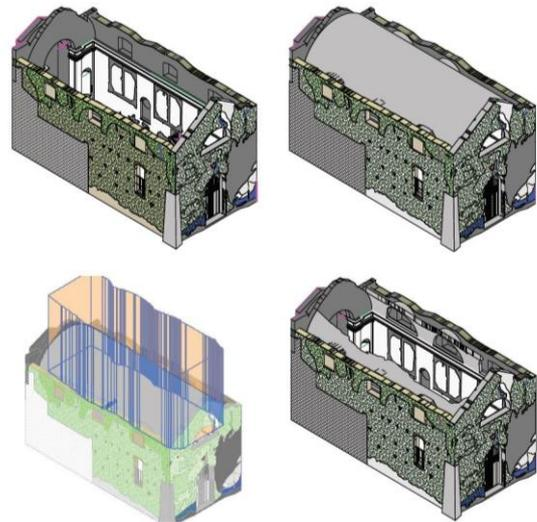
**Fig. 5:** Construction’s process of vaulted roof of the oratory
