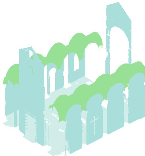
**Fig. 5** Wall, floor, and vaults segmented via RANSAC
