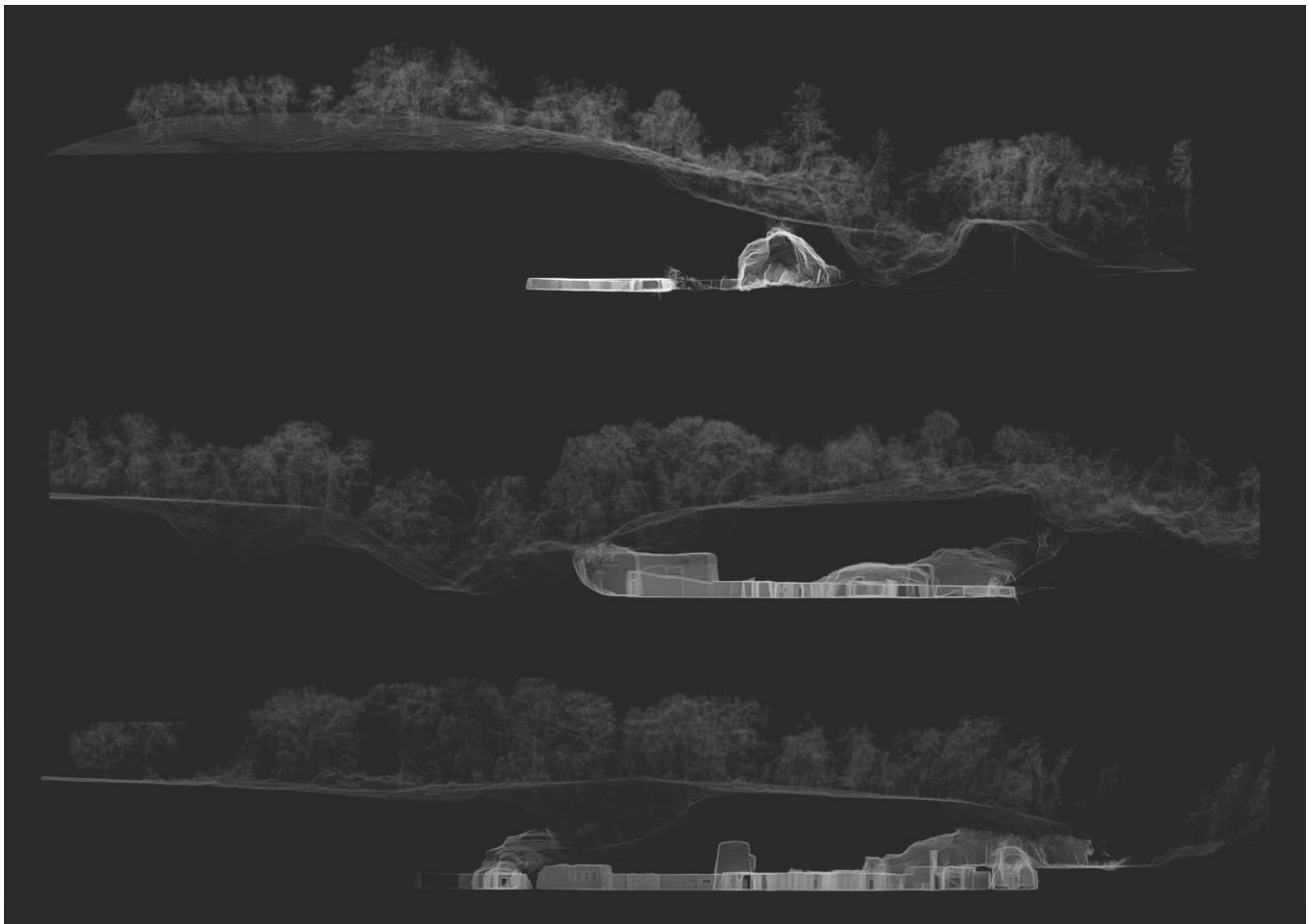
Fig. 16: Quarry point cloud sections visualized in PointCab (Source: authors' graphical elaboration).
