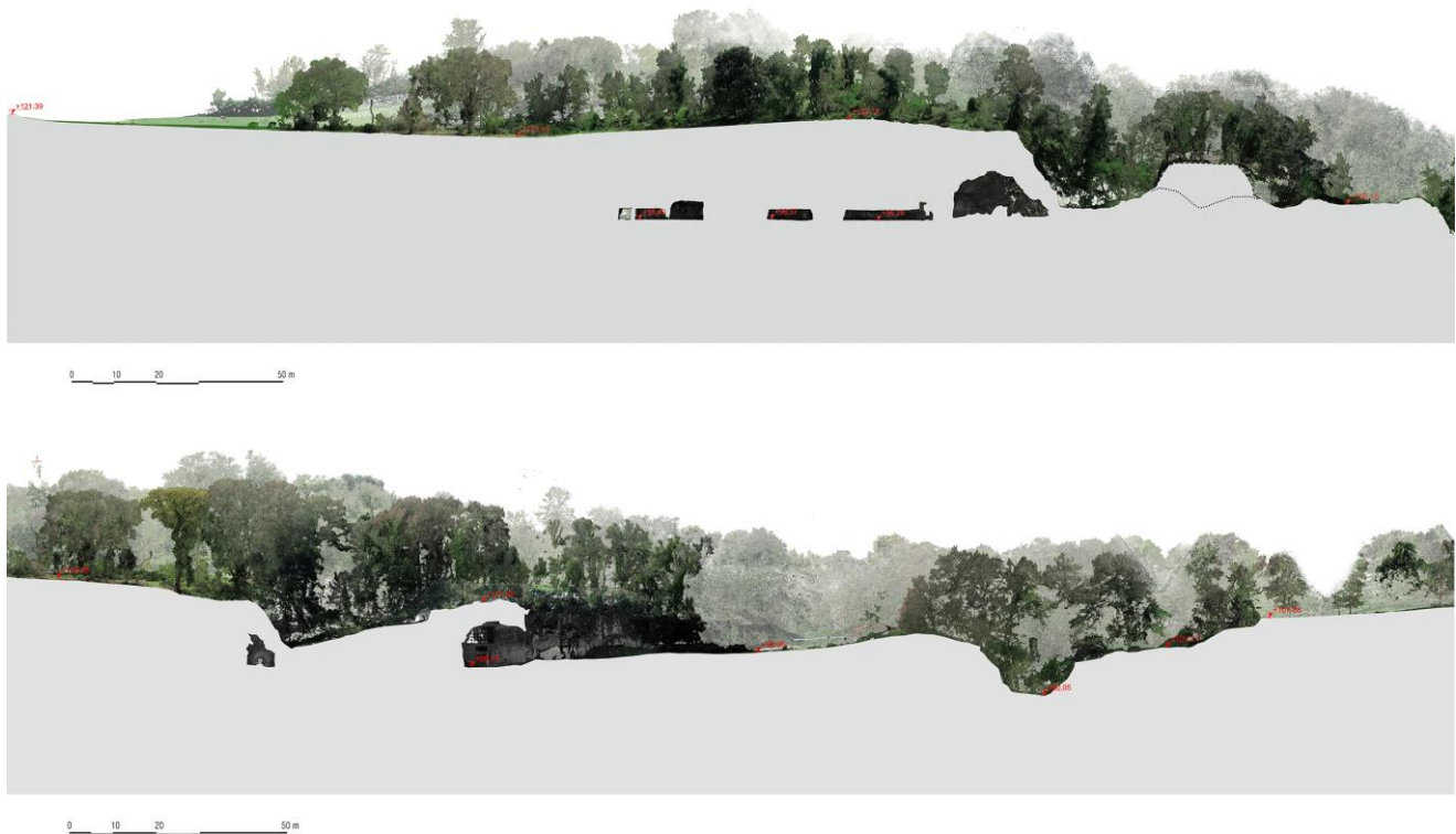
Fig. 18: Sections DD' and GG': orthophotomaps of the area obtained by integrating the LiDAR-based point cloud and the GeoSLAM point cloud, processed in CAD and Adobe Photoshop (Source: authors' graphical elaboration).
