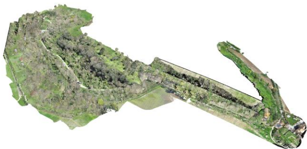
Fig. 10: Point cloud obtained from drone-based LiDAR acquisition visualized in RGB.
