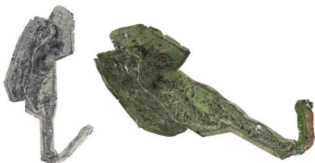
Fig. 13: Point cloud obtained from aerial photogrammetric acquisition (Source: authors' graphical elaboration).
