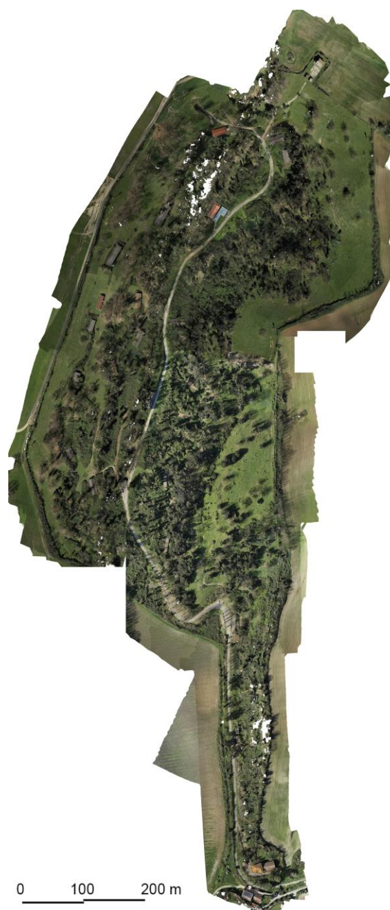
Fig. 12: Orthophotomap generated from aerial photogrammetric processing (Source: authors' graphical elaboration).
