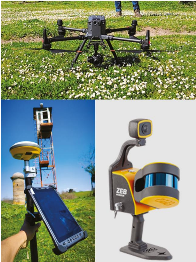
Fig. 4: DJI Matrice 350 RTK equipped with a DJI Zenmuse L1 LiDAR payload and a DJI Zenmuse P1 photographic payload; E-100 RTK GNSS receiver by e-Survey; GeoSLAM Zeb Horizon (Source: authors' photograph).
