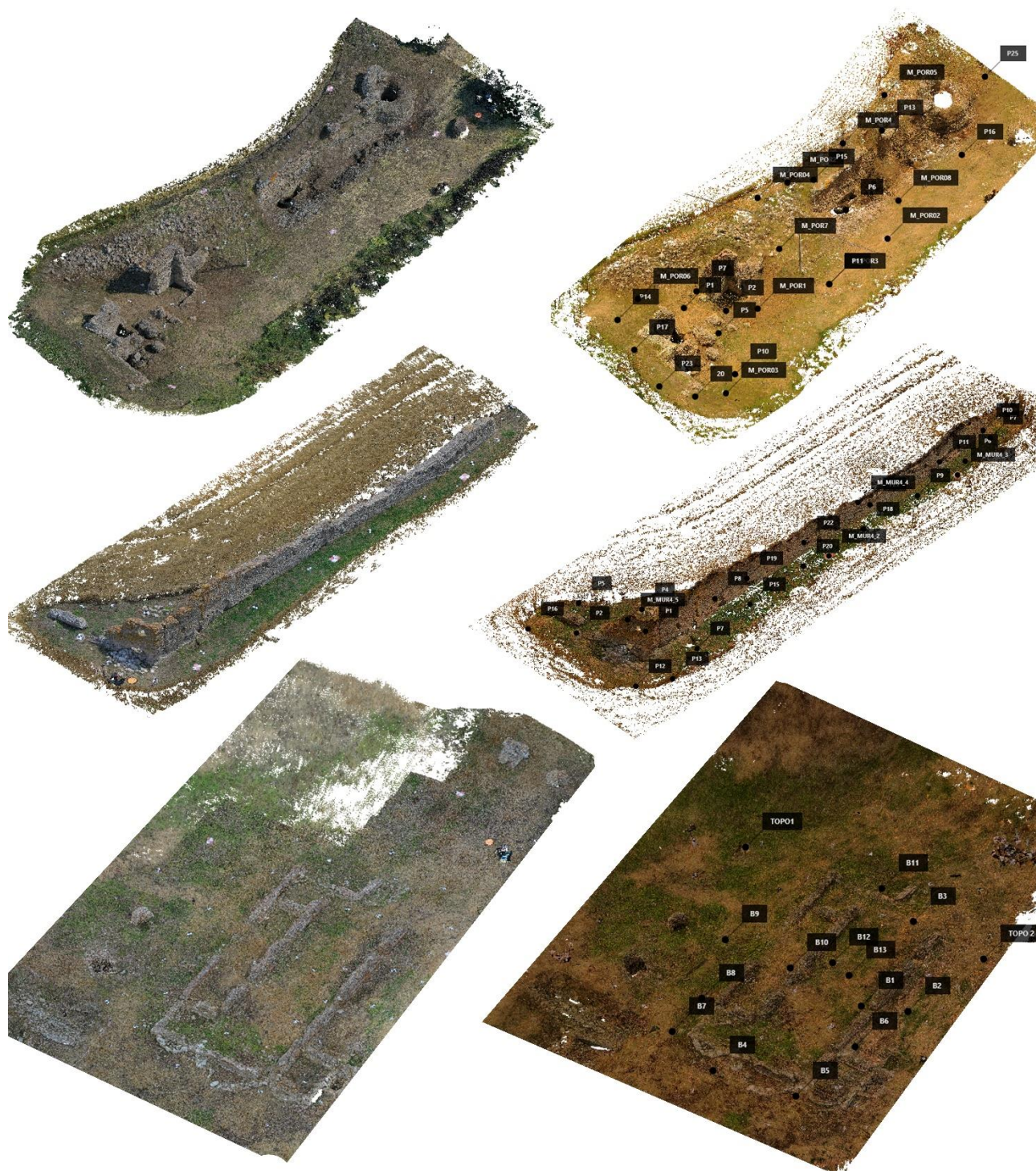
Fig. 13: Point clouds from laser scanner and photogrammetric survey: south-west gate, south-east wall, castellum
