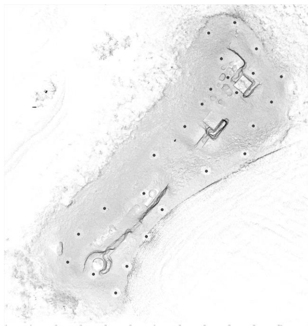
Fig. 10: Panoramic map processed with Faro Scene software showing laser scanner station points: south-west gate
