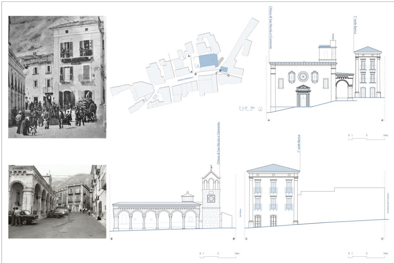
Fig. 12: Graphic elaboration of the premises of the Cooperative Bank resulting from integrated survey and comparative analysis with historical photographs.
