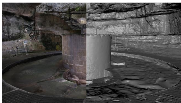
Fig. 8: Photogrammetric survey of Fonte Pliniano. The 3D approach guarantees great freedom in video shooting and the correct positioning of viewpoints in AR.
