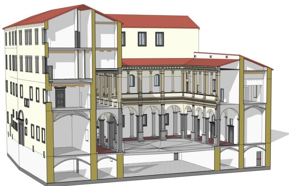
Fig. 3: HBIM model section of the former convent and the Chiostro of Santa Maria della Pace in Rome.
