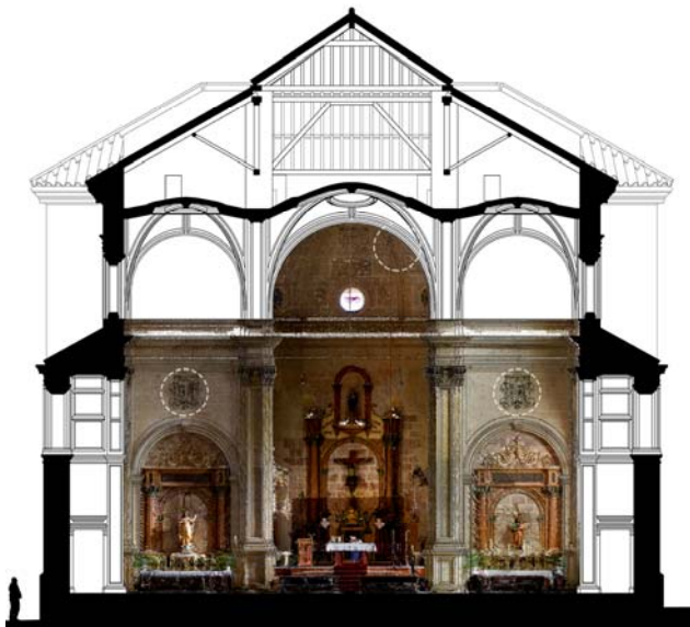
Fig. 4: Transverse section with the triumphal front highlighted, marking the cartouche dated 1558 and the coats of arms of Archbishop Pedro Guerrero. Own elaboration.
