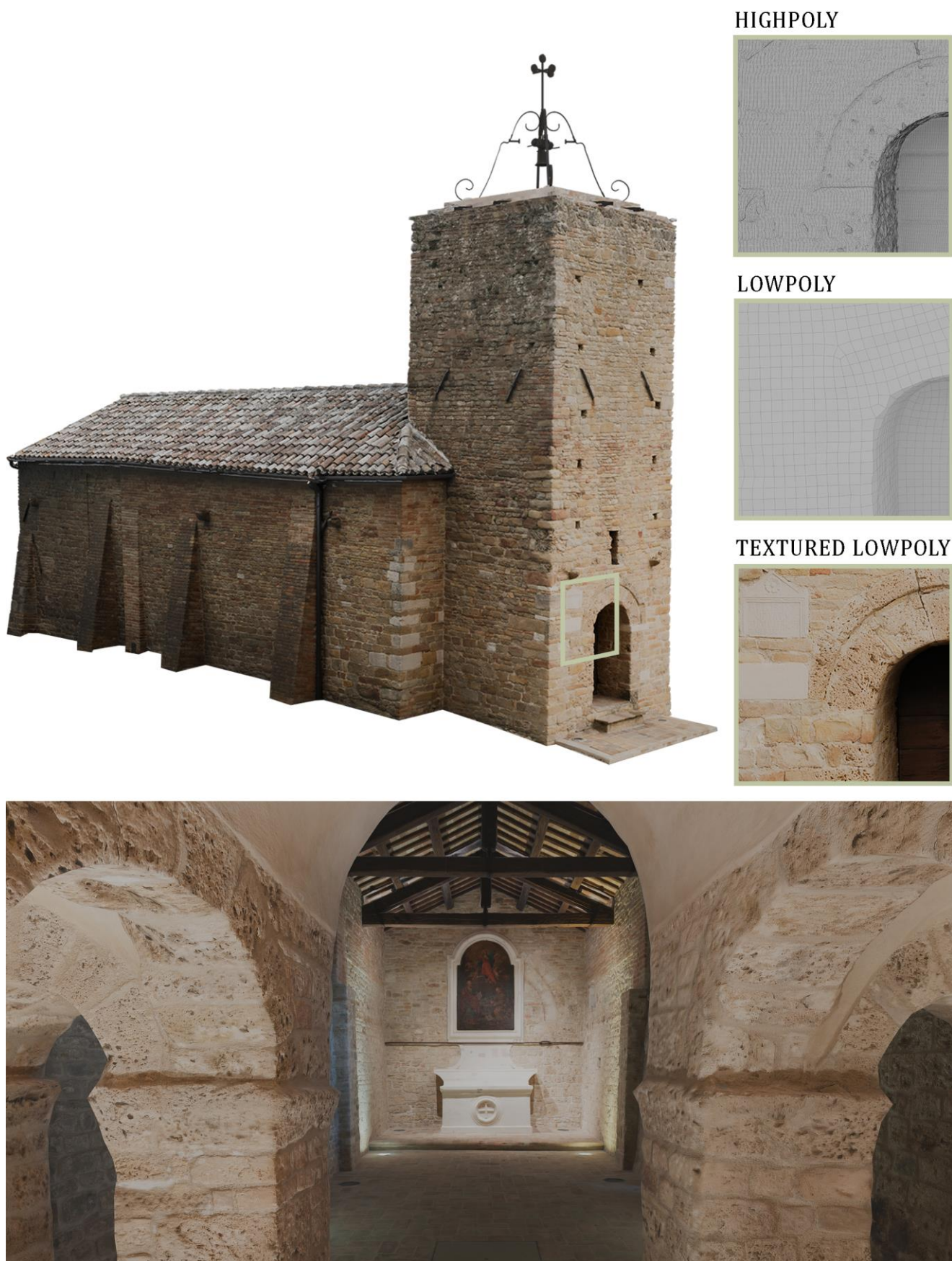
Fig. 3: External and internal views of the low-poly model after baking operations. Top right: detail showing a comparison between the high-poly, low-poly, and textured low-poly models.
