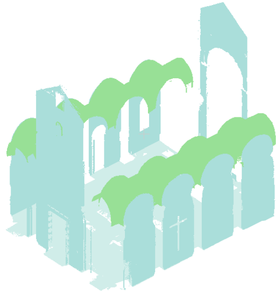
Fig. 5 Wall, floor, and vaults segmented via RANSAC
